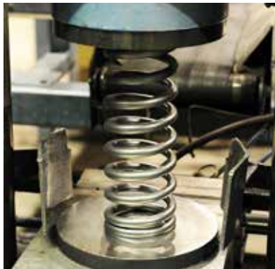
Fig 3. The presetting operation involves compressing the spring to implement a positive residual stress.
