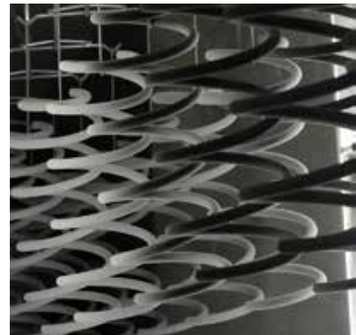
Fig 5. Coil springs being painted using an epoxy powder coating process.
