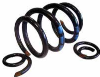
Fig 1. OE tapered wire spring with premature breakage at both end coils.
