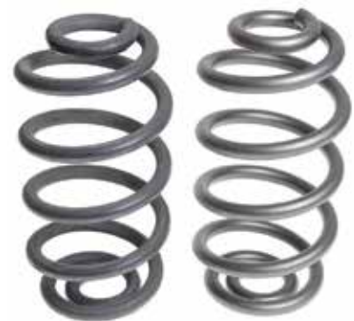
Fig 2. Coil springs before (left) and after (right) shot peening. Improved fatigue strength and an optimal paint surface.
