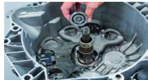
LuK RepSet® 2CT for the Renault 6-speed transmission (DC4) – the counter springs and lever actuators are tuned to work together at the plant, so they must be matched up correctly when installing the engagement system.
