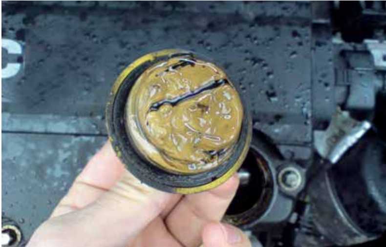
Warning sign: yellowish slime on the oil cap—an indication of condensate in the engine oil.
